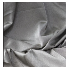
Silver-plated polyamide conductive fabric by 3L Tex
